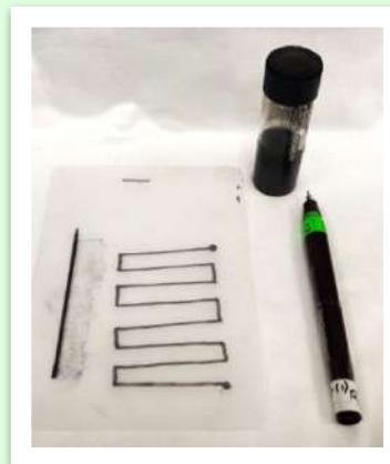
Natural rosin based conducting ink
