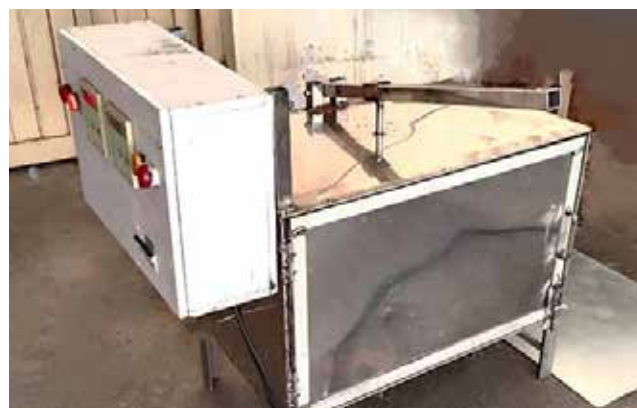
Melting behavior of hexagonal shaped seedlac under radiation heating at 300 °C & melt filtration unit
