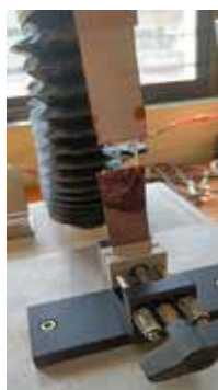
Pressure sensitive adhesives (a) Adhesive strength testing sunmica strips, (b) Adhesive strength of solvent-based formulations, and (c) Adhesive strength of aqueous formulations
