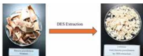
Cellulose extraction from banana pseudostem using DES
